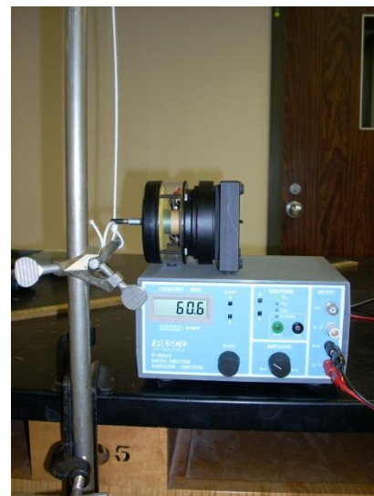
Figure 4. General layout of equipment for vibrating string.
